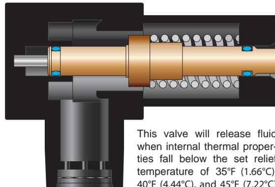
This valve will release fluid when internal thermal properties fall below the set relief temperature of 35°F (1.66°C), 40°F (4.44°C), and 45°F (7.22°C)
