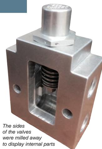
The sides of the valves were milled away to display internal parts
