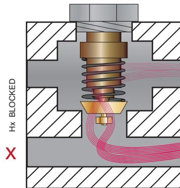
**Fig 3. DEMONSTRATES A HYPOTHETICAL SITUATION** WHERE THE COOLER IS BLOCKED CAUSING THE PRESSURE RELIEF FUNCTION TO BE ACTIVATED PREVENTING DAMAGE.
