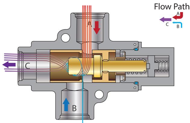
**Fig1:** Restricted cold flow into port B
