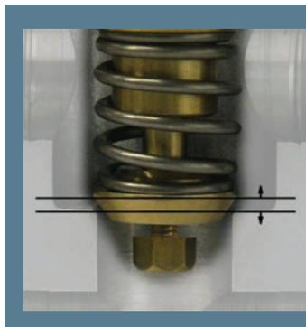
**Safety Pressure Relief:** Under normal pressure, the valve stays closed, directing the hot fluid to be cooled by the heat exchanger. Excessive pressure pushes up on the valve, compressing the spring and allowing fluid to flow straight out of the system without being directed by the heat exchanger. When the valve is closed, it sits at the bottom line. Excessive pressure pushes the spring to move the valve to the upper position pictured in the diagram.
